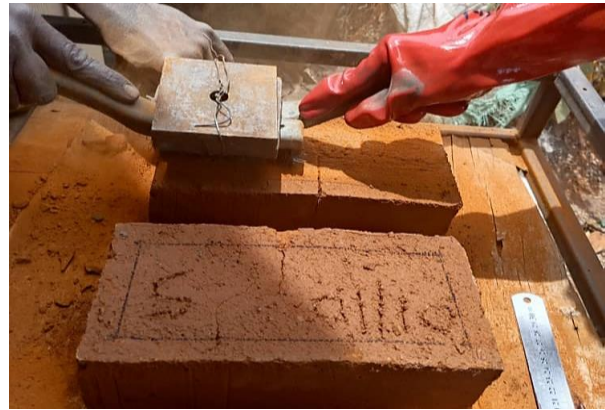
Figure 3: Abrasion test on a block
