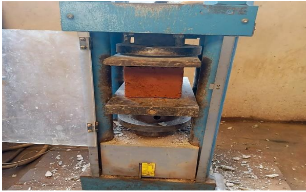
Figure 2: Compressive test on a block
