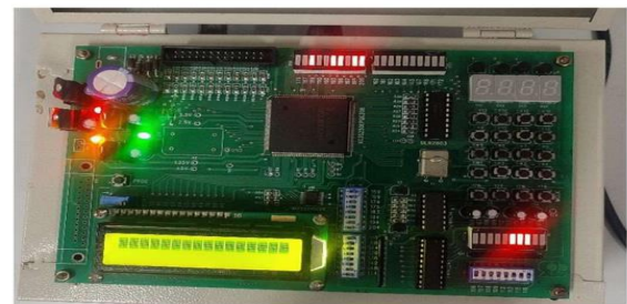
Figure 9. Output of Wallace Tree with Compressor in Spartan 3E FPGA board
