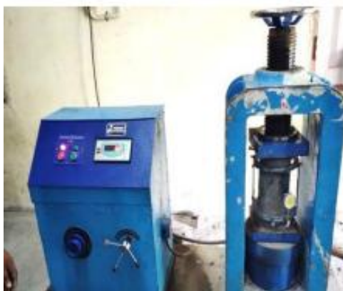
Fig.10 Elasticity Modulus Test
