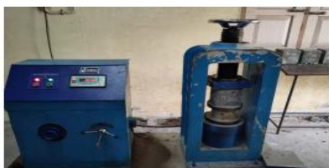
Fig .7 Cube Compression Strength Test
