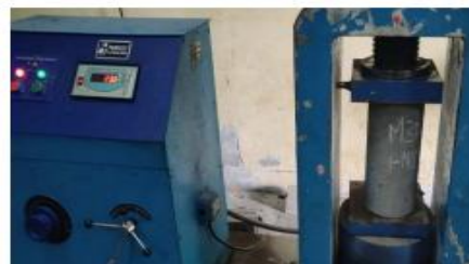
Fig.8 Cylinder Compression Strength Test
