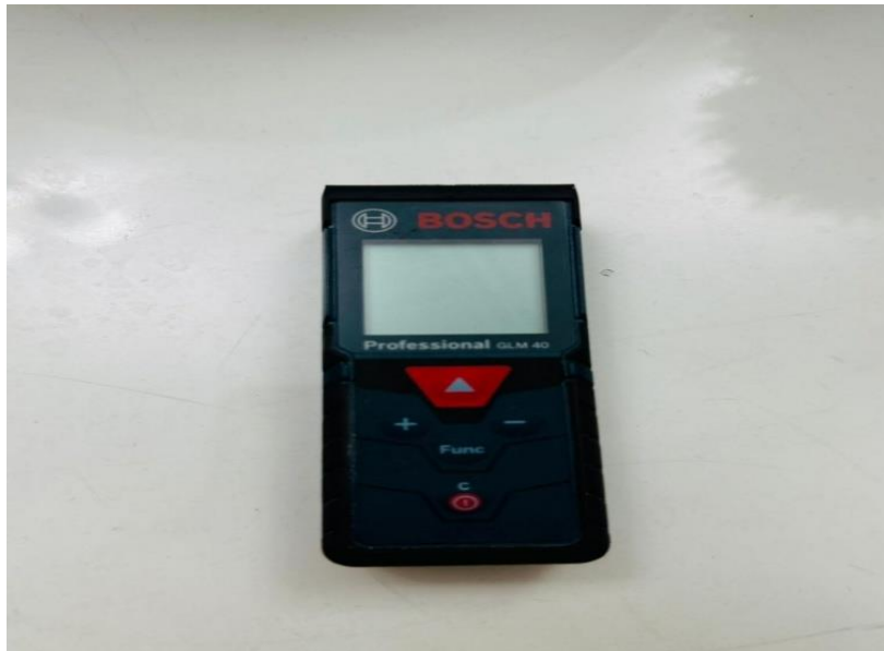
Fig 3: Bosch GLM 40 Distance Meter
