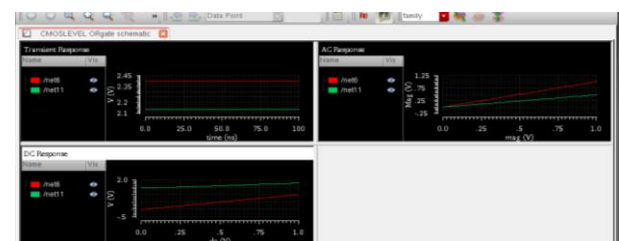
Fig. 3. schematic and output analysis of exclusive-OR gate using CMOS technology
