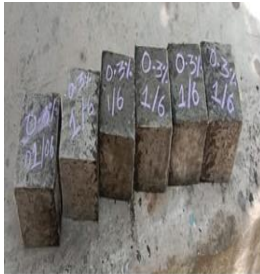
Figure 2. Specimen for Compression Test
