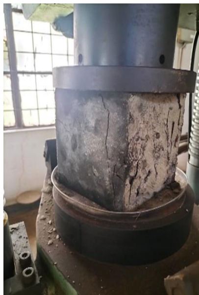
Figure 2. Specimen for Compression Test
