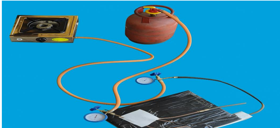
Figure 3: Experimental Setup of LPG-Based Refrigeration System with Pressure Gauges and Evaporator Unit
