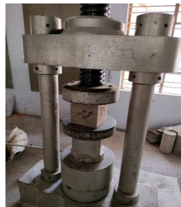
Figure 2. Compressive Testing of Cube Specimen
