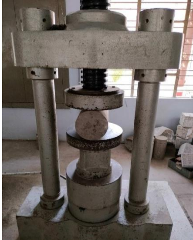
Figure 3 Split Tensile Testing of Cylinder Specimen
