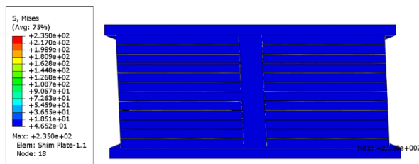
Figure 6: Maximum Stress Contours Model LCLRB
