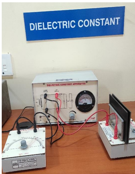
Fig.8 Experimental setup used for the measurement of the dielectric constant
