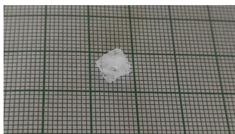
Fig.1. As grown 4-Chloro-N-(3,4-methylenedioxybenzyl)-aniline (CMA) crystal
