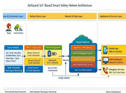
Fig. 2. Air Guard's system architecture showing sensor integration, data processing, and multi-channel communication pathways (Bluetooth, Wi-Fi, GSM).
