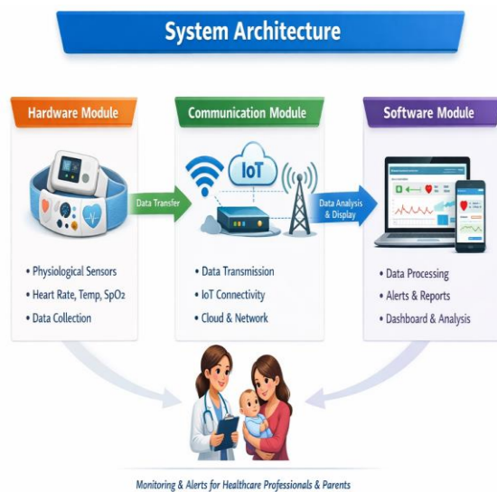
Fig 2: Overall System Architecture of the Proposed Infant Monitoring System
