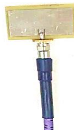
Figure 13. Fabricated patch antenna with SMA and coaxial connection for signal transmission.
