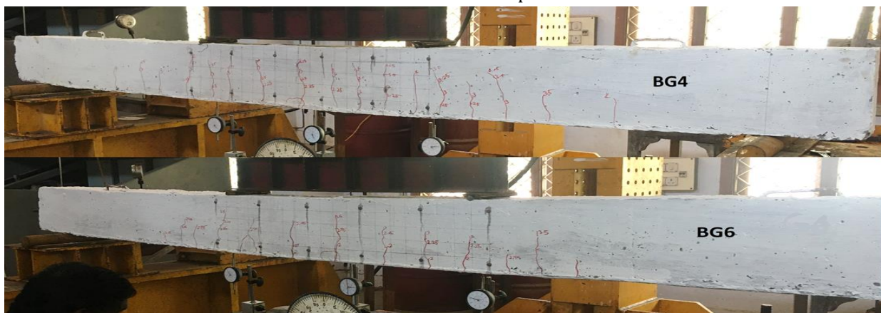
Figure 9 Failure of TRM strengthened Beams
