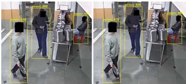
Figure 4. Real-time detection performance comparison. (Left) YOLO pre-trained model; (Right) YOLO custom-trained model
