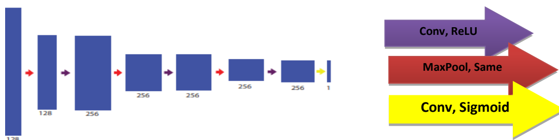
Figure 4: The discriminator block diagram as a decoder
