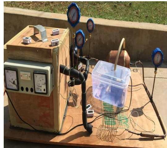
Fig 2: Experimental set up/Test Rig with shell & Tube condenser
